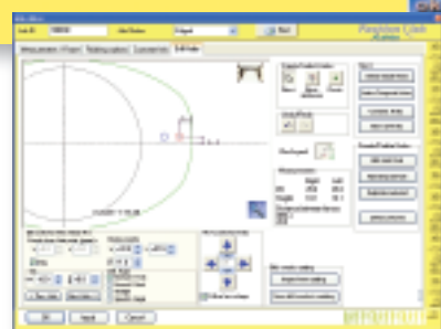
Figures 4 and 5 With this software (Fashion Lab, Activisu), customized rimless lens design is possible. Lens shapes are superimposed over a digital image of the patient's face. Both the lens size and shape can be edited while maintaining the drill hole and optical center. Also included is an integrated database which stores shapes, drilling points, and patient data. (Figures courtesy of Santinelli International, distributor.)
