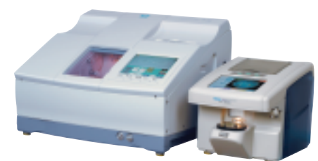
Figure 3 Many core technologies are available in a stand-alone format, such as this multifunction edger (ME-1000, Nidek), left, which provides 3D drilling and grooving capabilities, and this tracer/blocker (ICE-9000, Nidek), right.
