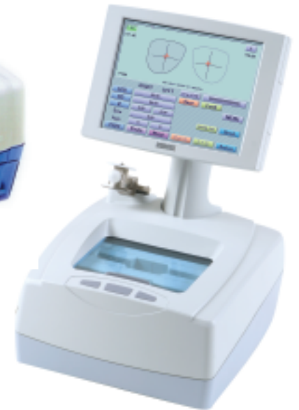
Figure 1 (top) This frame tracer (LT-900, Nidek) can send frame and patient data directly to an off-site wholesale lab.
